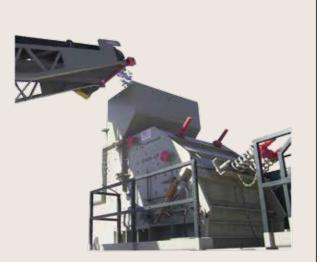
Feeding method is critical with an impact crusher. Optional feed chute designs allow the impactor to be fed from three sides with a stacking conveyor.
